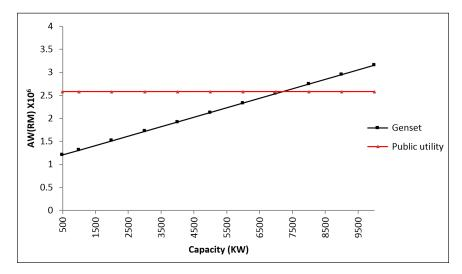
Figure 14. Effect of capacity on redundancy evaluation
