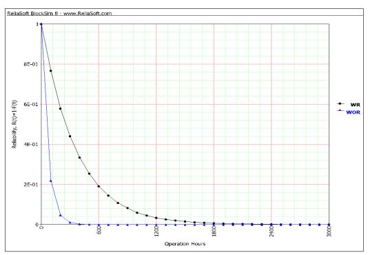
*Figure 5.* Binary system reliability of power generation system with redundancy (WR) and without redundancy (WRO)
