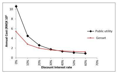
Figure 15. Effect of interest rate on redundancy evaluation
