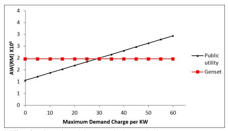
Figure 13. Effect of maximum demand charge on redundancy evaluation
