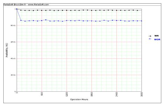
*Figure 4*. Binary system availability of power generation with redundancy (WR) and without redundancy (WRO)
