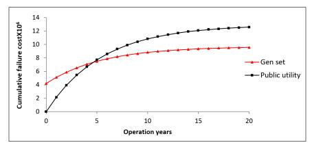
Figure 11. Comparison of Gen set and public utility based on failure cost evaluation
