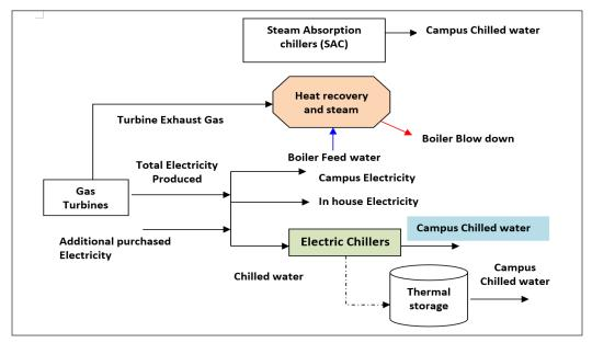
Figure 2. System configuration of cogeneration
